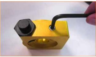
5. Remove any excess Teflon® after tightening.
