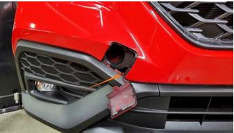
**02.** Using a 19mm socket and driver, install the threaded rod into the tow hook hole. Tighten to 20 lb-ft.
