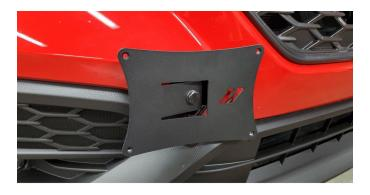
**05.** Using a 4mm allen wrench, attach your license plate to the license plate mounting bracket with the (4) M6 bolts.
