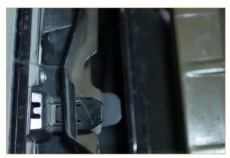
26. Remove the ten grille clips from the vehicle and transfer them to the grille for reinstallation. To remove the clips, squeeze the tabs together and extract the clip from the radiator support. To install the clips on the bumper, slip the head of the clip through the slot in the bumper, and twist the clip to seat the tabs into the channel on the back side of the bumper. (10x grille clips)
