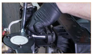
20. Loosen the two clamps that secure the cold-side intercooler pipe to the intake and the intercooler. Then remove the cold-side intercooler pipe. (2x 11mm T-bolt clamps)
