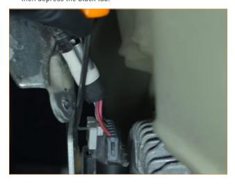
12. Remove the bolt that secures the fan clutch harness secures the retainer for the and then remove the retainer. (1x 10mm bolt)
