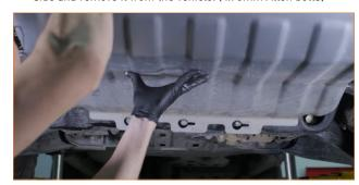
**03.** Remove the four tree clips that secure the air diversion panel to the underside of the fan shroud. (4x tree clips)
