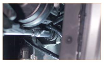
28. Remove the two bolts that secure the intercooler to the radiator support. (2x 14mm bolts)
