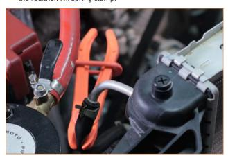
Now repeat this process on the lower transmission cooler line. (1x spring clamp)
