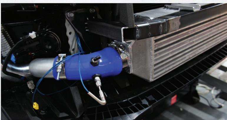
**Figure 3: Mounting location for Inlet temperature sensor, which reads approximately 10 times per second.**
