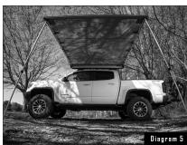
**17.** Secure the awning to the horizontal support arms using the Velcro tabs.
