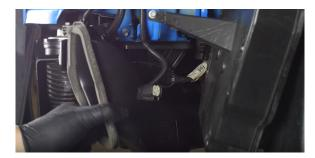
12. Loosen the clamp securing the hot-side pipe to the intercooler end tank. Then, separate the connection. (1x worm gear clamp)
