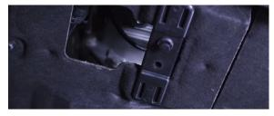
Remove the undertray by unscrewing the rest of the hardware securing it. (8x T30 torx screws, 2x pop-clips)
