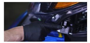
3. Remove the pop-clips that secure the undertray to the stabilizer bar. (2x pop-clips)
