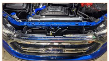
02. Remove the radiator grille. Loosen the two bolts at the top of the grille, then pull forward to disengage the tabs along the bottom and side edges.
