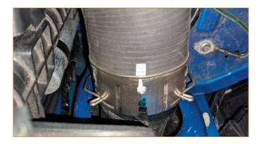
18. Loosen the worm gear clamp at the throttle body.
