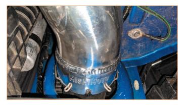
21. Install the cold-side silicone coupler with 2x high-torque worm gear clamps packaged in a separate polybag. Adjust the silicone hose, pipe, and clamps following the same procedure as step 13. Fully tighten all clamps.
