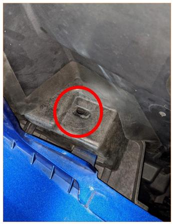
**08.** Remove the painted bumper fascia and the black plastic support bracket assembly from the vehicle. Start at the corners of the bumper fascia, pull to disengage the tabs along the underside of the headlights.
