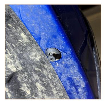
**05.** Carefully pull back the front part of the fender flare to expose the hex head bolt underneath, then remove the bolt.
