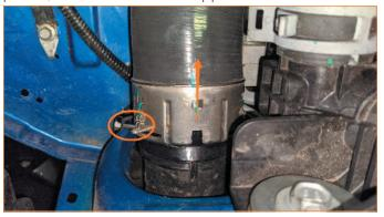
05. Loosen the worm gear clamp at the turbo side.
