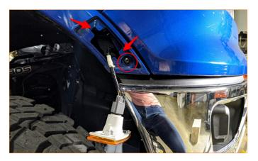
**04.** Remove the pop clip closest to the truck's front end that secures the fender flare to the wheel well liner.
