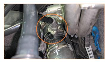
**17.** Disconnect the cold-side pipe from the intercooler following the same procedure as step 4.
