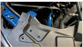
02. Loosen 2x worm gear clamps, disconnect the vacuum line and tree clip at the back of the intake hose, then remove the rubber intake hose.
