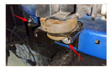
13. To install the Mishimoto intercooler, reverse the stock intercooler removal procedure. Note that the Mishimoto intercooler includes 4x shorter M5 bolts to install the top trim piece to the intercooler and a longer M5 bolt for the MAP sensor to replace the stock hardware.
