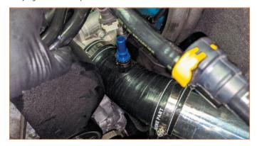
**22.** Connect the vacuum line with the blue fitting on the cold-side silicone hose. The cold-side intercooler pipe install is now complete.
