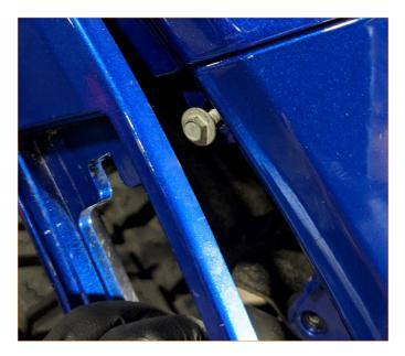
**06.** Remove 3x bolts securing the bumper fascia support (black plastic structure) to the frame, along the intercooler's underside. Repeat steps 3–6 on the other side.
