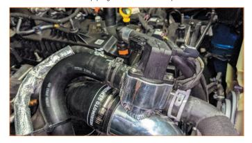
**16.** Disconnect vacuum fitting from the stock cold-side (driver side) pipe, close to the throttle body.
