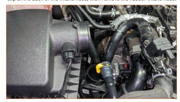
03. Unbolt the stock hot-side (passenger side) intercooler pipe from the engine block. (1x 13mm bolt)
