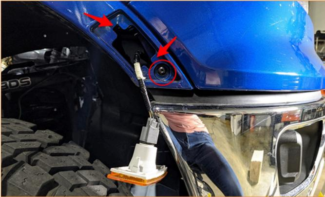
**04.** Remove the pop clip closest to the truck's front end that secures the fender flare to the wheel well liner.
