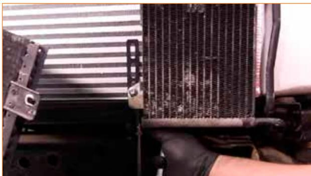
12. Attach the transmission cooler to the driver-side end tank of the intercooler with the supplied bolt, but do not fully tighten it yet. (1x 10mm bolt)
