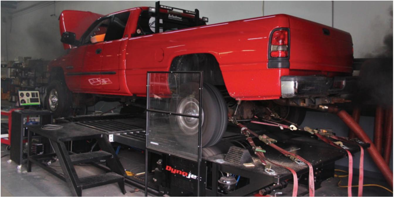
FIGURE 6: Dynamometer testing of the Mishimoto Intercooler
