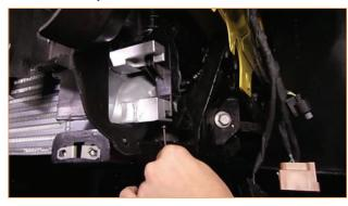
**28.** Tighten the worm-gear clamp on the hot-side pipe. Make sure that the boot is seated all the way on the intercooler. (7mm socket, 7mm socket wrench, or flathead screwdriver)
