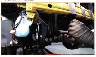
**7.** Separate the clip to free the air shutter arm.
