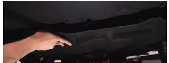
8. Remove the final plastic under-panel that's directly under the front bumper. (4x T30 torx)
