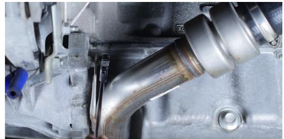
2. Loosen the clamp on the coupler between the hot-side pipe and turbo.
