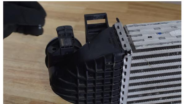
24. Install the sensor removed from the stock end tank onto the Mishimoto intercooler. Secure it with the bolt from your kit. (1x T25 torx bolt)
