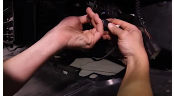
17. Squeeze the four tabs to release the bumper guard.
