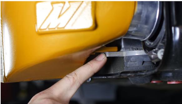
26. Secure the intercooler to the lower mounts using the original bolts. (2x 8mm bolts)
