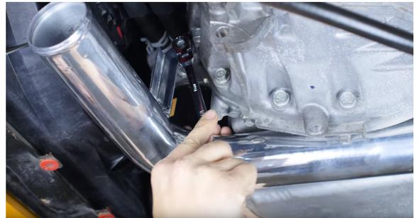
7. Slide two clamps over the larger coupler in your kit. The longer end of the coupler will attach to the hot-side pipe and the shorter end goes to the intercooler. (2x worm gear clamps)
