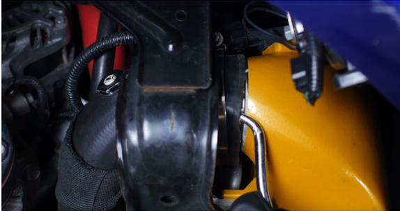
12. Loosen the clamp securing the stock cold-side pipe to the throttle body. Pull down on the pipe to separate it from the throttle body, and then lower it from the vehicle. (1x worm gear clamp)
