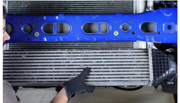
23. Remove the sensor from the end tank on the stock intercooler. (1x T25 torx screw)
