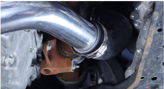
6. Align the pipe so it will fit in the crease between the transmission and oil pan without touching either. Rest the two brackets welded to the pipe on the studs you removed nuts from earlier. Secure the pipe with those original nuts. (1x 10mm nut, 1x 13mm nut)
