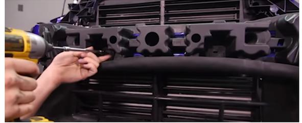
16. Disconnect the electrical connector for the active grille shutters, and then pull out the tree-clips holding the wire. (2x tree clips)
