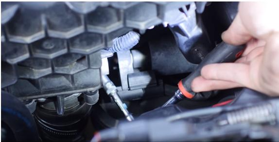
13. Slide a clamp over each end of your Mishimoto cold-side pipe. We recommend tightening the clamps enough so they sit on the coupler and do not move out of position. (2x worm gear clamps)
