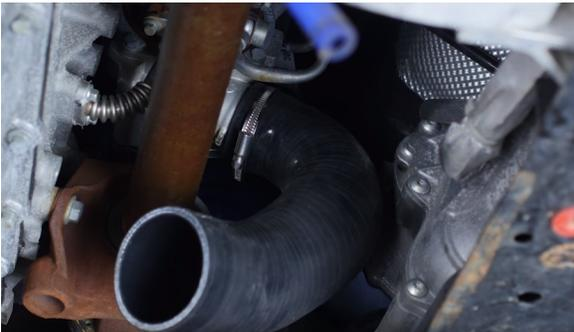
5. Install the intercooler pipe to the open end of the coupler you just installed to the turbo. (1x worm gear clamp)
