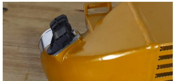
25. Install the Mishimoto intercooler, making sure as you lift it into position to slide the tabs on the radiator into the upper intercooler hangers. Then, push the bottom of the intercooler forward and allow it to sit on the mounts.
