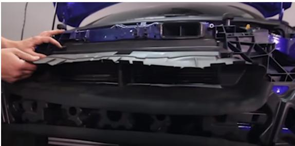
15. Remove the lower air shroud, which is held by two screws.
