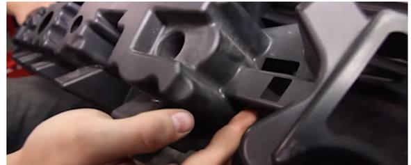
18. Loosen the clamps on the cold- and hot-side pipes connected to the intercooler. (2x worm gear clamps)
