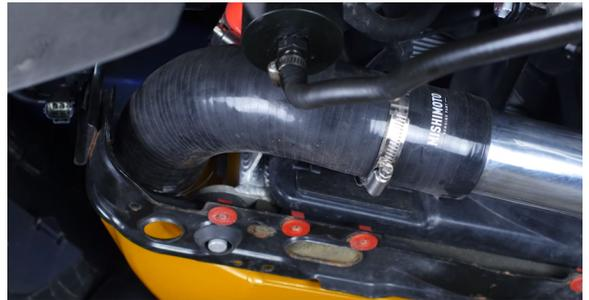
9. When tightening the second clamp, make sure it is over the pipe's bead roll. Do the same with the clamp securing the connection between the first coupler and hot-side pipe.
