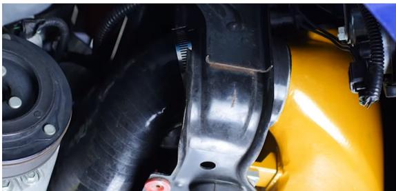
15. Rotate the coupler up and install it onto the throttle body.
