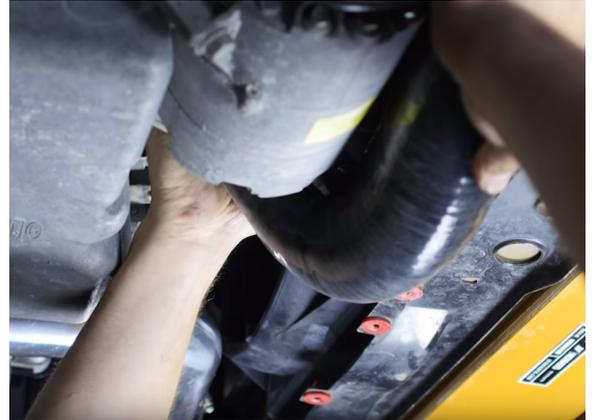
16. Tighten each clamp, making sure that the coupler is fully seated and the clamp isn't on the bead roll of either port. Reinstall the engine cover.
