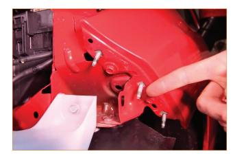
Remove the bumper cover by sliding it forward, away from the vehicle.
