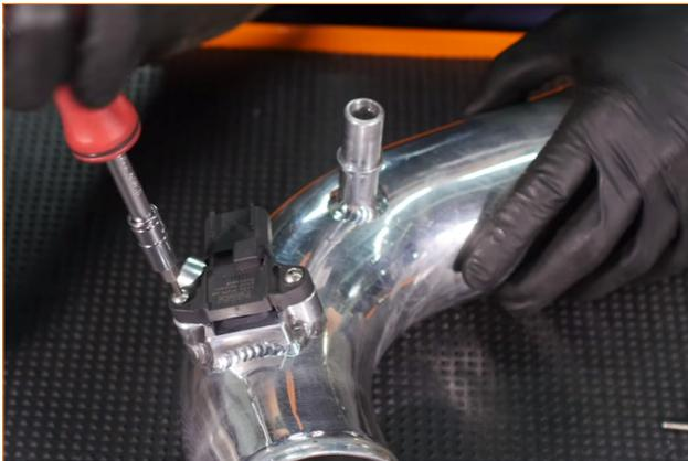
42. Locate the last coupler in your kit. One side of this coupler is larger than the other. The wider end of the coupler gets an 86–94mm clamp, while the smaller end gets a 79–87mm clamp. Install the clamps, and then attach the smaller end of the coupler to the upper section of the cold-side pipe. Slide it all the way until the pipe protrudes from the coupler. (2x T-bolt clamps)
