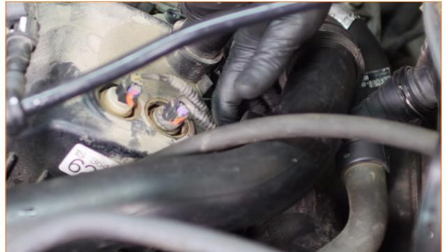
15. This system has a lot of couplers and pipes to be installed. Pay special attention to the orientation of the clamps to make sure the adjustment nuts will be accessible when the pipes are installed. Leave all the clamps loose until the pipes are fully assembled to allow for adjustment.
