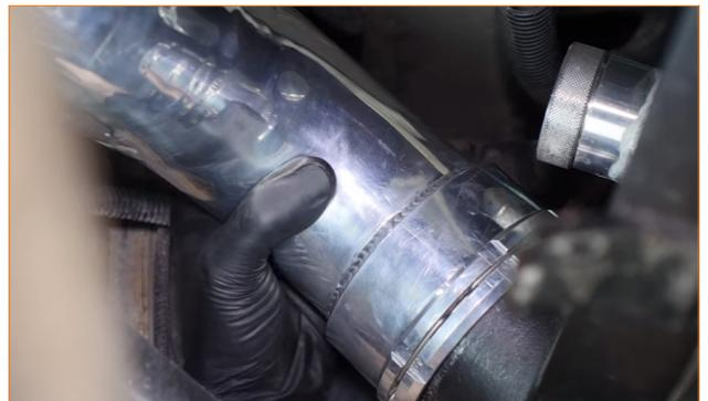
38. Locate the transition coupler included with your kit. Install an 89–97mm clamp over the wider end of the coupler and a 79–87mm clamp over the smaller end.
