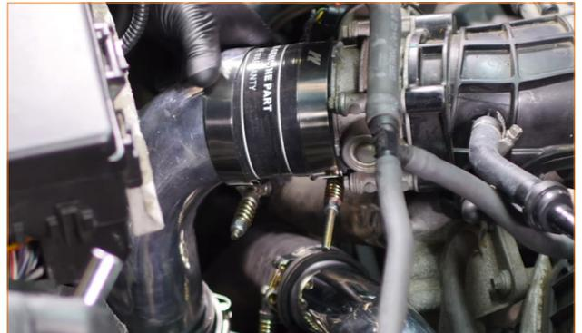
44. Check to make sure that the transition coupler is positioned over the bead roll of both pipes, and tighten the clamps to secure it.
