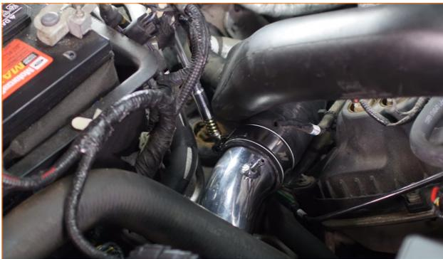
33. Reconnect the hoses to the passenger-side induction pipe and intercooler pipe.
