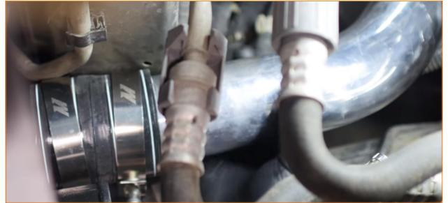
28. Align the driver-side intercooler pipe with the lower inlet of the intercooler, and slip the coupler down to join the connection.
