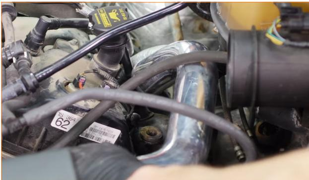
19. Locate the single-bend, long coupler included with your kit. Identify the smaller end of the coupler and install a 63–70mm clamp over this end. Then lower the coupler into place and slip it over the pipe you just installed. (1x T-bolt clamp)
