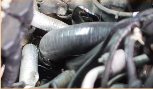
24. Locate one of the 67–75mm clamps in your kit and slip it over the end of the coupler you just installed. (1x T-bolt clamp)
