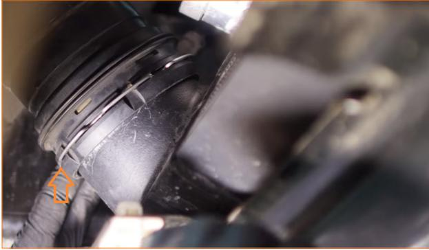
12. Loosen the clamps that secure the hot-side pipes to the intercooler. Then wiggle the pipes to break them loose from the intercooler. (2x worm gear clamps)
