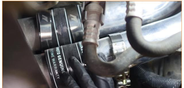
29. Make sure the couplers are fully seated over both pipes and the intercooler inlets, and then tighten the clamps that secure the couplers to the intercooler. Leave the clamps on the pipe side loose for now so that you can adjust the position of the pipes.
