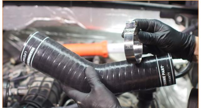
20. Locate one of the 67–75mm clamps included with your kit and slip it over the coupler you just installed. (1x T-bolt clamp)
