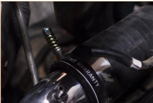
26. Locate the last coupler in the hot-side pipe kit and assemble it just like the last one. The smaller end gets a 67–75mm clamp while the larger end gets a 73–81mm clamp. (2x T-bolt clamps)
