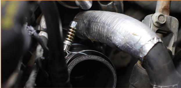
18. Locate the upper section of the driver-side intercooler pipe. Lead the end with the shorter run of pipe underneath the hoses at the front of the engine bay, and turn the pipe so that the other end runs across the front of the engine. Then slip the pipe into the coupler at the turbocharger.
