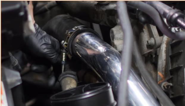
32. Tighten the clamp that secures the passenger-side turbocharger coupler to the intercooler pipe. Then secure the passenger-side induction pipe to the engine by pushing the pin on the pipe into the grommet on the engine.
