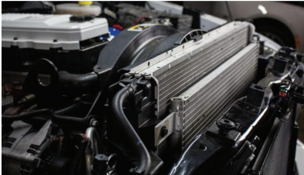
**FIGURE 1:** *The stock 2015-2018 Dodge RAM 6.7L Cummins transmission cooler mounted in the truck.*
