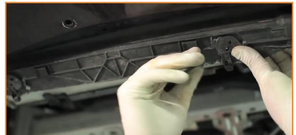
5. Remove the bolts on the intercooler. This will allow you to remove the intercooler from the engine bay. (2x T25 torx bolts)
