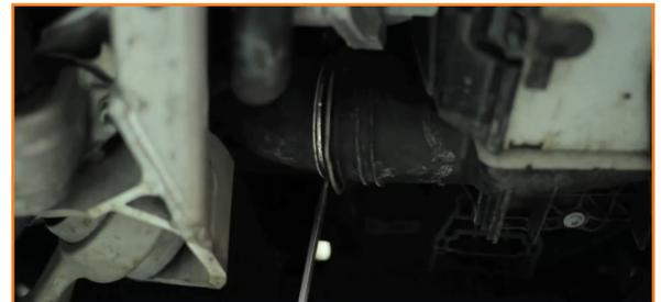
4. Turn the tabs on the intercooler shrouding to release it from the intercooler.
