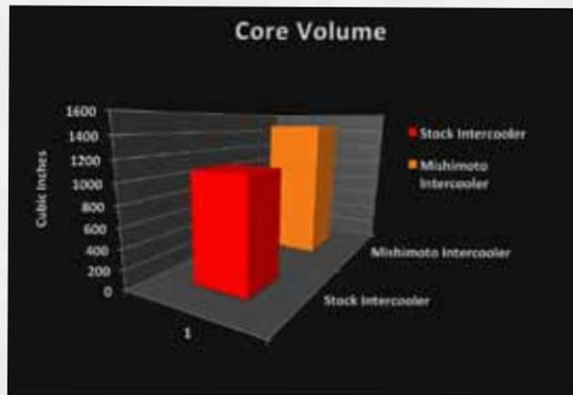
The engineering team went through multiple iterations while designing the end tanks. They used CFD software to make sure that the flow was optimized for the Chevrolet/GMC 6.6L Duramax. The core of the Mishimoto intercooler is 23% thicker and 25% larger in volume than the stock unit.
