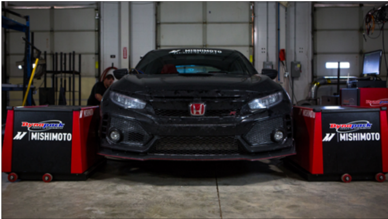
FIGURE 7: A Dynapack dynamometer was used for vehicle testing.
