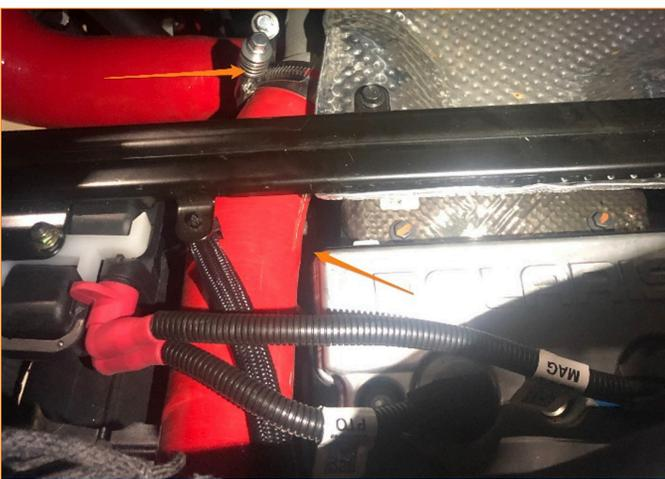
11. Using a T-20 Torx, remove the MAP sensor from the outlet side of the factory charge pipe. Install the MAP sensor in the sensor fitting of the charge pipe. Secure with the provided bolt using a 3mm allen key. The MAP sensor fitting may need to be adjusted slightly by rotating it in place. Re-install MAP sensor and throttle body electrical connections.
