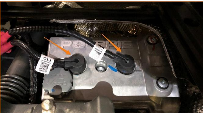
06. Loosen the 2X T-bolt clamps holding the factory charge pipe to the turbo outlet and the throttle body. Loosen until the nut reaches the end of the T-bolt for easiest removal.
