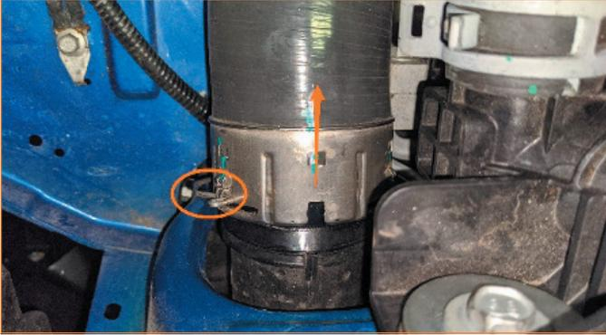
**05.** Loosen the worm gear clamp at the turbo side.
