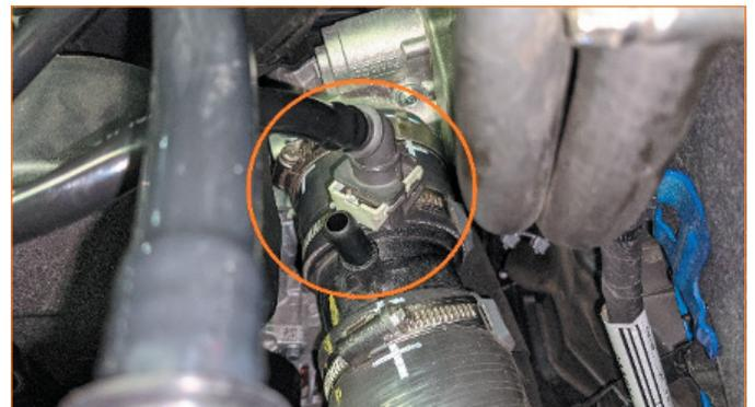
**17.** Disconnect the cold-side pipe from the intercooler following the same procedure as step 4.
