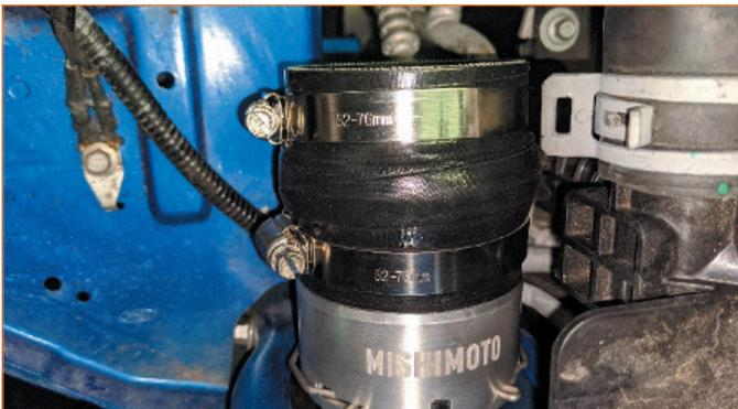
**12.** Install the aluminum pipe section and secure it to the engine block with the original 13mm bolt you previously removed. Do not fully tighten.
