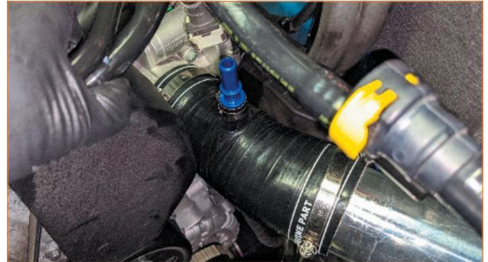
22. Connect the vacuum line with the blue fitting on the cold-side silicone hose. The cold-side intercooler pipe install is now complete.
