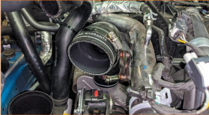
**11.** Install the short silicone coupler with 2x larger clamps left in the 4-clamp polybag. Leave the clamps loose.
