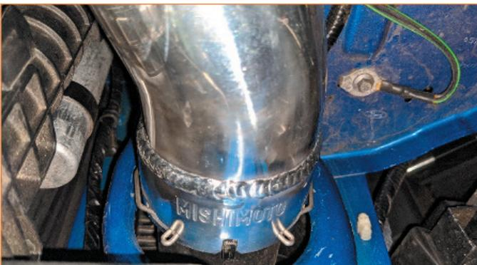
21. Install the cold-side silicone coupler with 2x high-torque worm gear clamps packaged in a separate polybag. Adjust the silicone hose, pipe, and clamps following the same procedure as step 13. Fully tighten all clamps.
