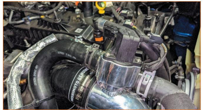
**16.** Disconnect vacuum fitting from the stock cold-side (driver side) pipe, close to the throttle body.
