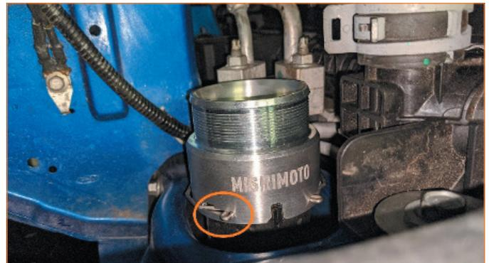
**10.** Install the turbo-side silicone hose with 2x high-torque worm gear clamps. Locate the polybag with 4x clamps; the single smallest clamp goes on the turbo end of the hose. Leave the clamps loose.
