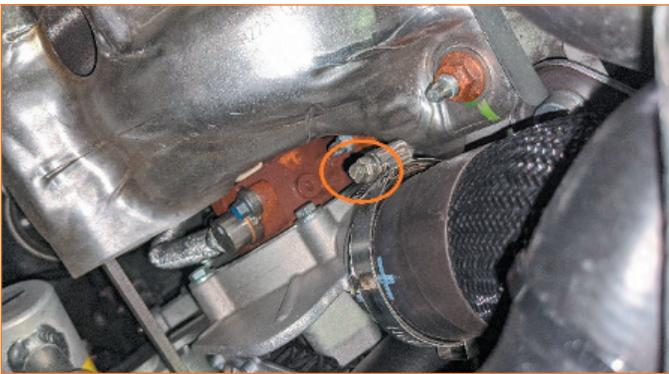
**06.** Unplug and remove the blow-off valve from hot-side pipe. (3x 8mm plastic screws, 1x tree clip)
