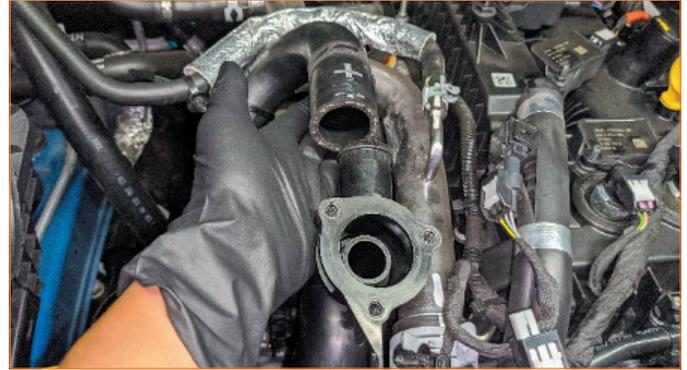
**08.** Remove the stock hot-side pipe assembly from the vehicle.
