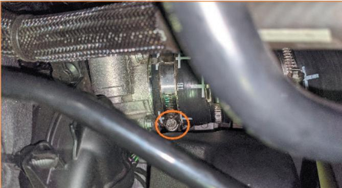
19. Remove the stock cold-side pipe assembly from the vehicle.
