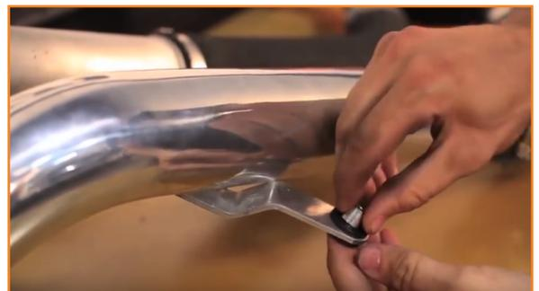
14. Install couplers to the intercooler pipes. (2x T-bolt clamps)
