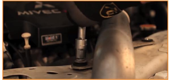
11. Loosen the clamp where the upper intercooler pipe meets the intercooler. Slide the pipe off the intercooler end tank.
