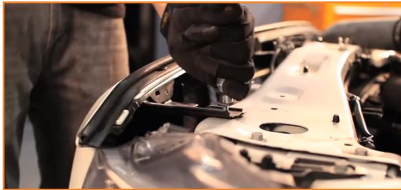
8. Remove the bolts on the front grille mounting points. Next, disconnect the fog light harness and remove the hardware. (2x 10mm bolts, 1x pop-clip)
