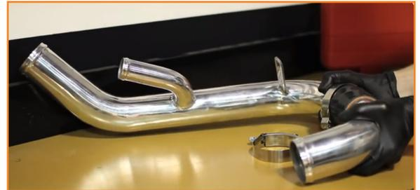
20. Install the pipe along with one of the included couplers to the intercooler. (2x T-bolt clamps)
