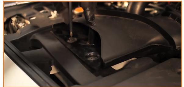
5. Remove the bolt that secures the airbox. Loosen the clamp where the intake hose meets the airbox. Then remove the airbox from the engine bay. (1x 10mm bolt, 1x 10mm clamp)
