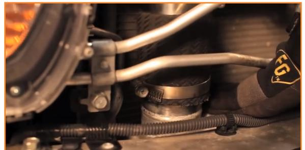
12. Loosen the intercooler pipe from the turbo inlet, and then slide the pipe off the turbo.
