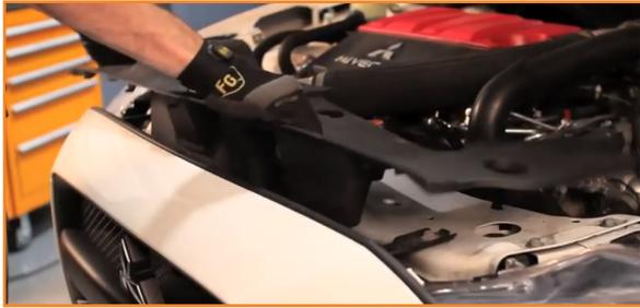
7. Unbolt the front bumper from the support bracket. (5x 10mm bolts)
