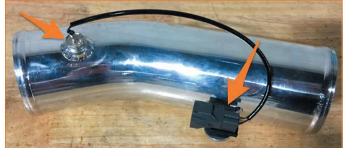
17. Remove the temperature sensor from the stock cold-side pipe and install it into MM2364-01. [1x temperature sensor and 1x harness tree-clip]
