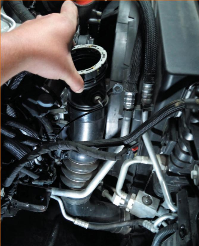
16. Remove the stock cold-side pipe from the vehicle.
