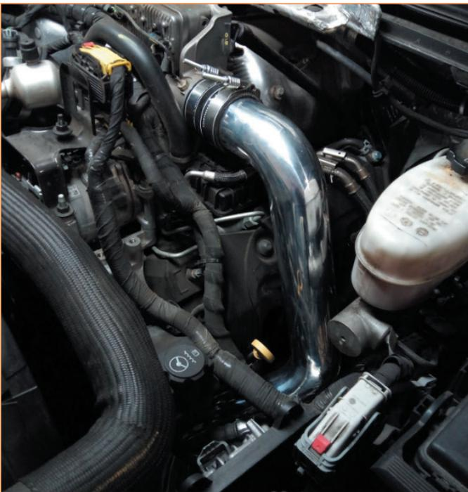
**05.** Connect MM2365-01 and MM4124-03 to the turbo outlet using the provided constant tension T-bolt clamps, leave the clamps loose. (1x MM1331-3 and 1x MM1331-325)
