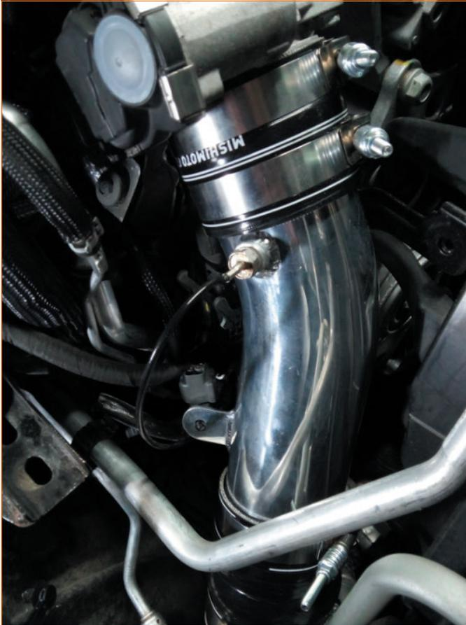
20. Connect MM2364-01 to the intake manifold using MM4549-01 and the provided constant tension t-bolt clamps, leave the clamps loose. [2x MM1331-35]
