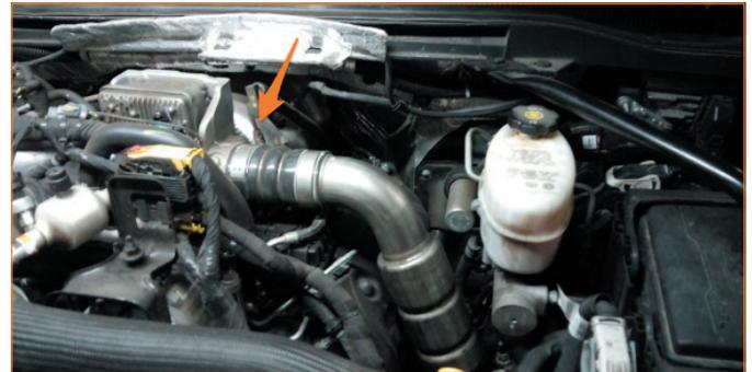
**02.** Loosen the constant tension T-bolt clamp securing the stock hot-side intercooler pipe to the turbo outlet. (1x T-bolt clamp)
