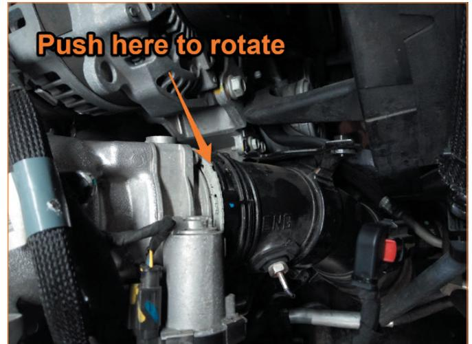
**15.** Remove the stock cold-side intercooler pipe from the intake manifold. (1x plastic locking ring)
