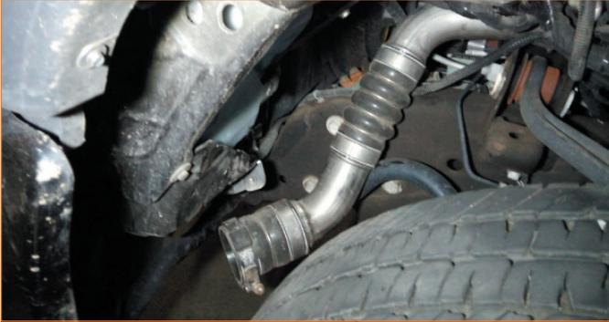
**04.** Remove the stock hot-side intercooler pipe through the driver-side wheel well.
