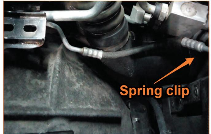
**14.** Remove the stock cold-side intercooler pipe from the intercooler. (1x spring clip)
