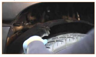
**5.** Remove the mounting plate for the airbox by removing the four 10mm bolts.
