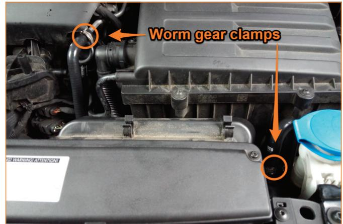
3. Route the Mishimoto coolant hose under the air box ducting, then secure it in place using the provided worm gear clamps.
