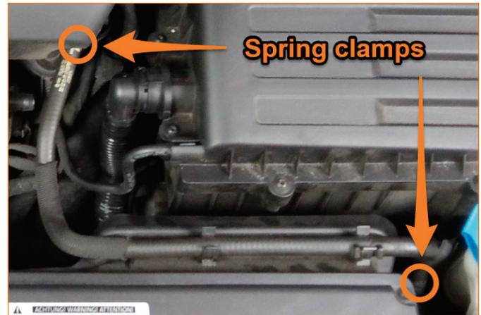
2. Remove the stock coolant hose from the driver side of the radiator. (2x spring clamps)
