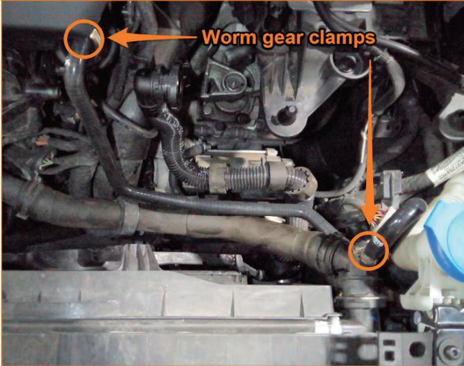
\*The image above shows the Mishimoto coolant hose routing with the air box removed\*
