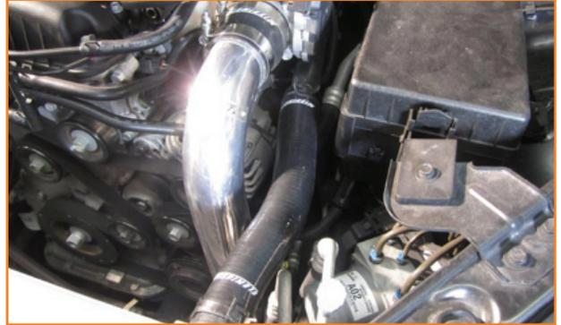
3. Reinstall and tighten the negative terminal of the battery. Refill coolant, check for leaks, and bleed out air by turning the vehicle on and squeezing the upper and lower radiator hoses.
