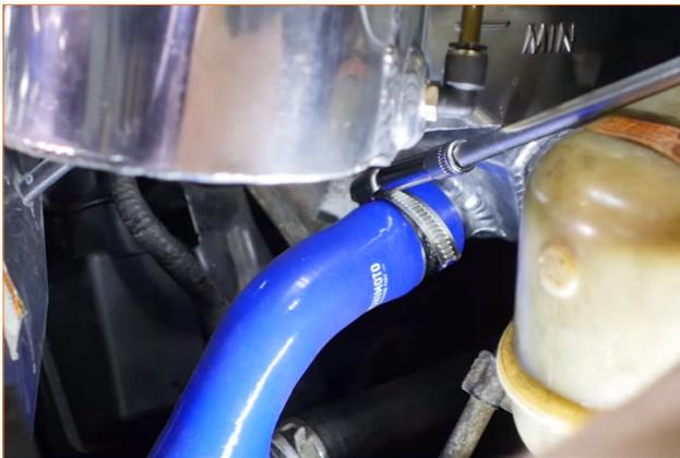
24. Secure the expansion tank to the firewall with the two original bolts. (2x 8mm bolts)
