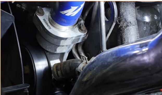
14. Install the provided worm gear clamps over each end of the Mishimoto lower overflow hose. (2x worm gear clamps)
