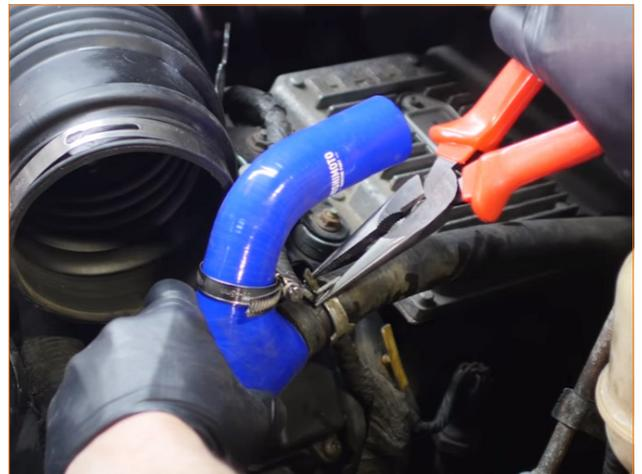
17. Go back and tighten the clamp that secures the lower overflow hose to the front cover. Check to make sure that the hose clamp will not interfere with the belt or pulley.
