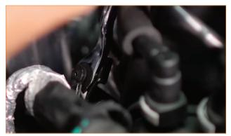
**09.** Separate the two tree-clips that secure the heater hoses to the engine. Then separate the upper heater hose from the water pump. (2x tree-clips)
