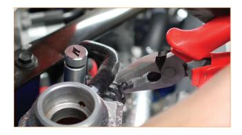
12. Separate the quick-disconnect fittings that secure the heater hoses to the firewall and remove the hoses from the vehicle. Each fitting has a clip that locks the hose in place. To release the fitting, the clip needs to be slid out until it snaps into the second detent on both sides. Use a pick and flathead screwdriver to release the clips. When you reinstall the hoses, simply lock this clip back into place to secure the hose.
