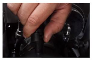
Loosen the two worm gear clamps securing the induction hose to the airbox and turbo. (2x worm gear clamps)
