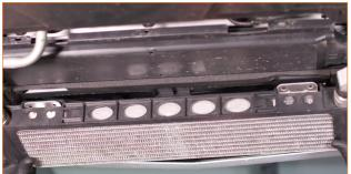
**09.** Place a drain bucket underneath the petcock on the radiator and use a pair of pliers to open the petcock. Remove the pressure cap from the expansion tank to expedite the draining process. Close the petcock on the radiator once all the coolant has drained.
