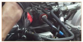
**23.** Compress the clamp that secures the overflow hose to the radiator and slide the clamp down the hose. (1x spring-clamp)
