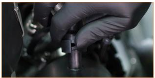
**04.** Disconnect the mass airflow (MAF) sensor and release the harness from the intake tubing. To release the connector, slide the red locking tab up, depress the black tab and pull the connector off the sensor.
