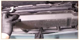
08. If equipped, remove the four nuts that secure the stock HD oil cooler to the underside of the vehicle. Slide the oil cooler off the studs to access the petcock on the radiator. [4x 10mm nuts]
