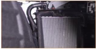
14. Place a drain bucket under the driver-side auxiliary (aux) radiator. Cut the zip tie that secures the protective sleeve to the inner hose. Compress the clamp that secures this hose and move the clamp down the hose. Remove the hose from the radiator. (1x worm-gear clamp)
