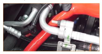
32. Lubricate the inside lip of each end of the upper radiator hose with fresh coolant and lower the hose into place. Lead the auxiliary radiator end of the hose first, passing it under the frame. Slip one of the provided worm-gear clamps over the radiator end of this hose and install the hose to the radiator. Repeat this process with the other two ends of the hose, and then tighten all the clamps. (3x worm-gear clamps)
