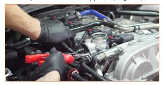
22. Compress the clamp that secures the overflow hose to the expansion tank and slide the clamp down the hose. (1x spring-clamp)
