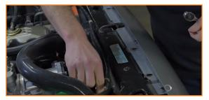
5. Detach the metal support just behind the grille's top edge. (4x 10mm bolts)
