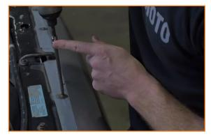
2. Remove the bolts that secure the upper support bar. You will need to remove the battery to reach one of the covered bolts. (6x 10mm bolts)
