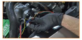
Cut the bullet connectors off the blue wire coming from each fan. Twist the two cut wires together. Put them inside the male spade connector and crimp the connector. Apply solder to the assembly.
