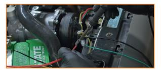
33. Run the black wire from the fan controller to the battery's negative terminal. Repeat previous steps for attaching a connector to this wire—strip, crimp, solder, and seal the assembly.
