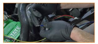
29. Run the provided red wire behind the battery to the positive terminal. The other end runs to the blue wire. Cut the excess wire.
