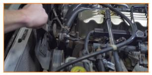
10. Remove the brackets that hold the AC condenser to the radiator. (2x 8mm nuts)
