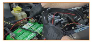
30. Strip both ends of the red wire. Crimp the shown connector onto one end. Apply solder and seal the connector using 1" of heat shrink.
