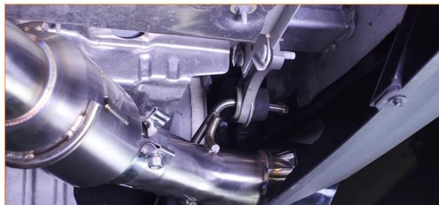
15. Snug the clamps between the tip assemblies and exhaust pipes.
