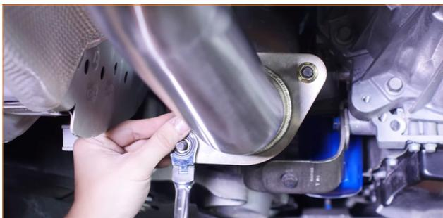
08. Slide a clamp over the front pipe you just installed. Then install the mid pipe over the open end on the front pipe. (1x exhaust band clamp)
