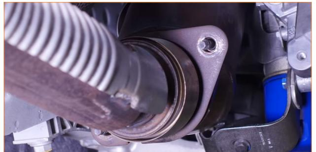
03. Use an exhaust hanger removal tool to pull the front bushing brackets from the exhaust hangers. Swing the bushing brackets to the side and out of the way once you've separated them. Repeat the process for the rear hangers.
