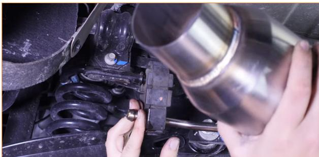
13. Organize the two exhaust tips in your kit so that they are positioned as though they were attached to the vehicle, each one with their hangers facing upward. Slide the driver-side and passenger-side brackets over the hangers on each tip assembly. The brackets are labeled, **Rear Face Right Hand** for the passenger side and **Rear Face Left Hand** for the driver side. Lubricate the rubber grommet on the bracket to help with this step.
