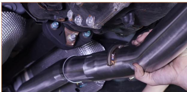
10. Slip the hanger on the rear pipe through the adjacent bushing bracket.
