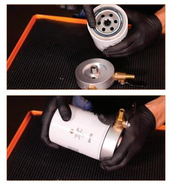
04. Install the mounting bracket to the filter housing. Orient the housing on the bracket as shown here. Install the three bolts, but do not fully tighten them yet as you may need to adjust the position later. (3x plastic washers, 3x 5mm Allen bolts)
