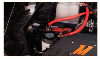
15. To replace the filter, move the valves to the closed position and unscrew the filter from the housing. Then install a new filter and turn the valves to the open position.
