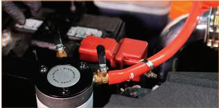
10. Locate the hose in your kit with a shallow bend. Install one of the small hose clamps over this end and slip the hose over the nipple on the EGR cooler. Install one of the large hose clamps over the other end of this hose and install it to the port marked IN on the filter housing. (1x small worm-gear clamp, 1x large worm-gear clamp)
