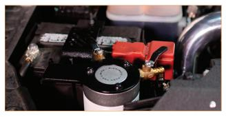
08. Compress the clamps that secure the EGR cooler hose and remove the hose. Place a cut-up bottle under the EGR cooler outlet to capture any spilled coolant. (2x spring clamps)
