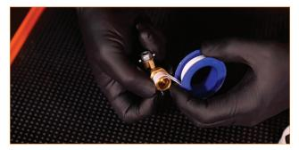
**02.** Install the ball values to the filter housing and tighten them completely. These fittings have a tapered thread so they may not be flush with the housing when fully installed.
