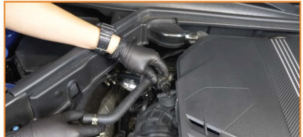
9. Install the open end to the outlet port on the catch can. (1x larger worm gear clamp)
