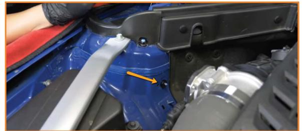
3. Loosen the nut on the passenger side strut tower, just above where you placed the spacer. Install the catch can bracket under the loosened nut as shown here. Secure the bottom of the bracket at the M6 stud. (1 x 10mm nut, 1 x 14mm nut)
