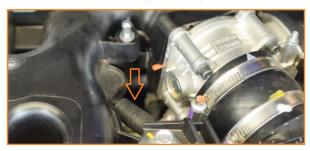
10. Attach the other end of the outlet hose to the catch can OUT port. (1x worm gear clamp)
