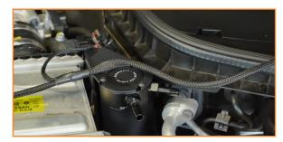
8. Remove the PCV hose. Compress the clamps on each end to free it. You will need to reach under and around nearby lines to get to the hose.
