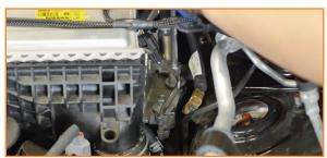
3. Install the catch can bracket to the intercooler bracket. Use the bolts you removed in the last step to secure the bracket. (2x 12mm bolts)
