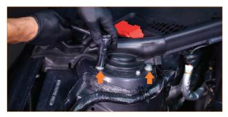
Remove the screw that secures the top of the heat shield below the passenger-side strut tower. (1x 10mm screw)
