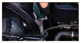
14. Lower the catch can assembly into place over the strut tower, and secure it with the hardware you just removed. Then go back and tighten the two bolts that secure the support strut to the catch can bracket. (2x 13mm bolts, 1x 10mm screw)
