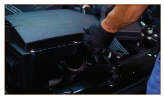
08. Locate the CCV hose attached to the front of the engine. Disconnect the hose from the valve cover by squeezing the tabs at the top of the hose and pulling the hose off. Then disconnect the wiring harness from the sensor at the other end of the hose. Separate the bottom of the hose by squeezing the tabs and pulling the hose off.
