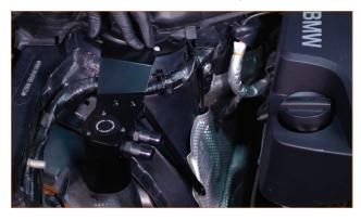
15. Locate the hose with the smaller bend, and install one of the provided hose clamps over the wider end. Install this end to the CCV fitting on the valve cover. Attach the other end of this hose to the fitting marked IN on the catch can. (1x worm-gear clamp)
