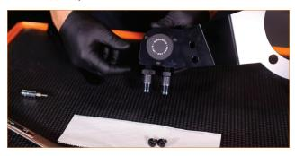
02. Install the two plastic fittings to the catch can and tighten them completely. Note that the threads on the fittings are tapered and will not be flush with the can when installed. (2x plastic fittings)
