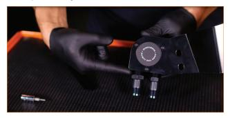
03. Attach the support strut to the bracket using the two provided bolts. Thread the bolts in, but do not tighten them completely. [2x 4mm Allen bolts]
