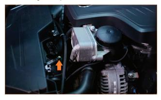
**07.** Remove the airbox from the vehicle by lifting it upward. The airbox is held in by three pegs and grommets.
