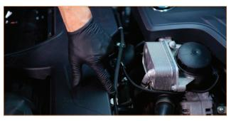
05. Disconnect the wiring harness from the mass airflow (MAF) sensor. To release the connector, depress the black tab.
