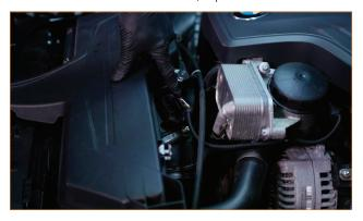
06. Loosen the clamp that secures the intake hose to the MAF housing. Then separate the hose from the MAF housing. (1x worm-gear clamp)
