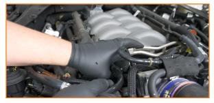
Remove the clips that secure the radiator cover. Once free, lift the radiator cover off the vehicle. (8x pop-clip)
