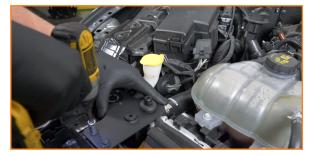
11. Connect the longer hose to the intake port on the engine and the outlet port on the catch can. (1x worm gear clamp)
