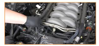
12. Connect the shorter hose to the PCV valve and inlet port on the catch can. (1x worm gear clamp)
