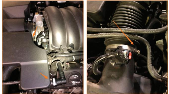
**02.** Remove factory PCV hose from the vehicle by pushing down on the white tab on the fittings while pulling on the hose. Use caution removing these components as they can be damaged with excessive force.
