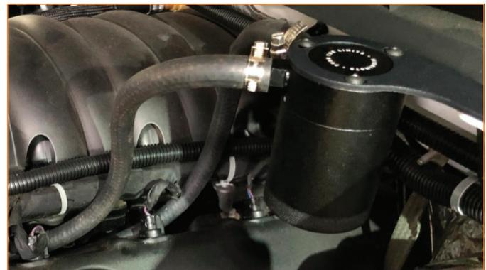
**07.** Adjust the orientation of the catch can and tighten the 3X 2.5mm allen head bolts.
