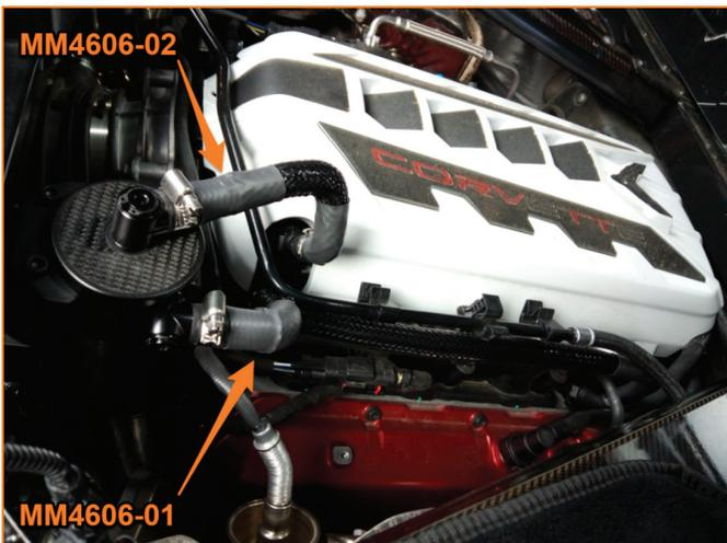
5. Secure the MM4606-01 hose to the EVAP line directly above it using the [2x MM1795-02 hose clips].
