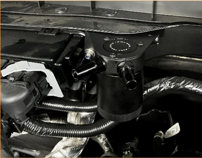
04. Attach catch can hoses as shown and secure with provided worm gear clamps.
