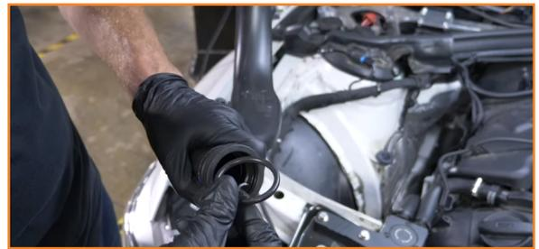
13. Attach a silicone coupler to the back intercooler pipe. Then set the back pipe on the turbo and slide the coupler onto the intercooler.
