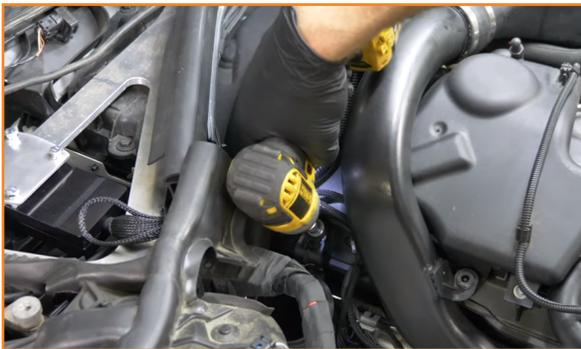
9. Remove the bolts that secure the intercooler pipes to the turbo. (2x E11 torx bolts)
