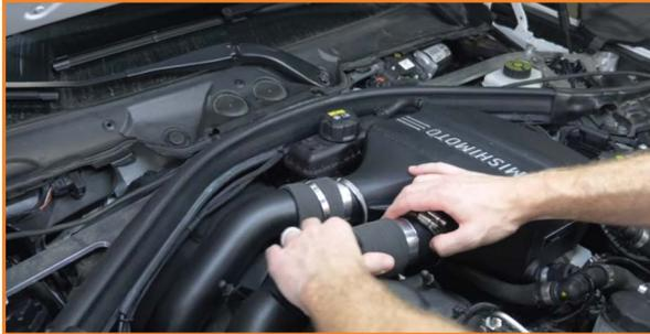
15. Tighten the clamps on both intercooler pipes.
