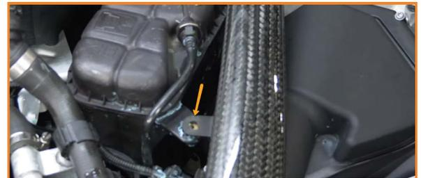
4. Slide the strut tower back to clear it from the engine bay.
