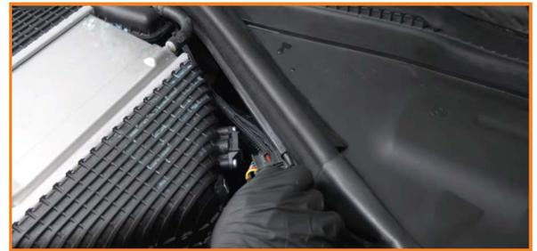
3. Loosen all the clamps on the intercooler pipes. (5x worm gear clamps)
