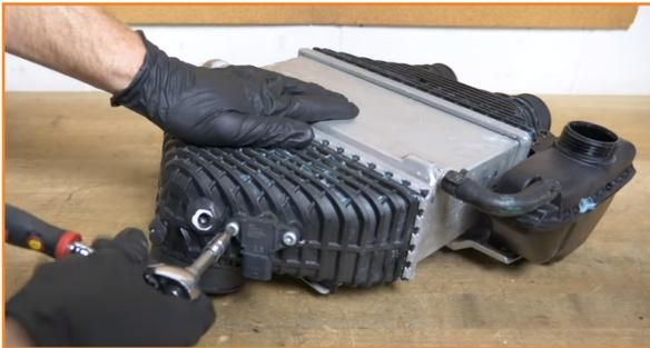
7. Compress the clamp on the small hose connecting the expansion tank to the intercooler. Slide the small hose off the intercooler port. (1x spring clamp)
