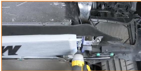
15. Remove the bolts on the lower part of the clam shell. (2x T25 plastic screws)
