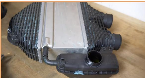
8. Detach the expansion tank from the intercooler.
