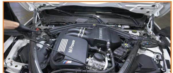
5. Lift the cover off the engine.
