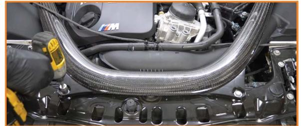
3. Remove the bolt that secures the primary expansion tank to the strut bar. (1x 10mm bolt)
