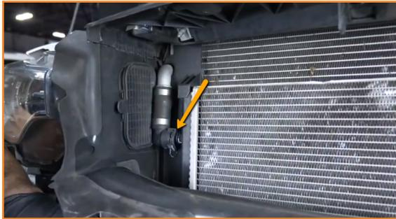
14. Remove the bolts that secure the oil cooler. (3x 13mm bolts)
