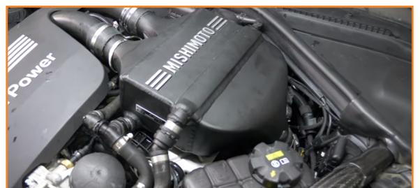
15. Reattach the quick-disconnects. (3x spring clips)
