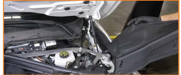
2. Remove the bolts that secure the front and ends of the strut bar. (8x 13mm bolts)
