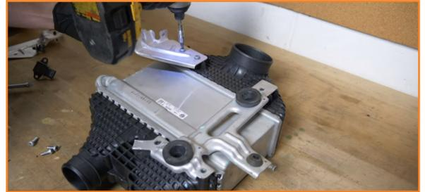
10. Transfer the brackets to the Mishimoto intercooler. Secure them using the provided hardware. (5x M5 3mm Allen bolts)
