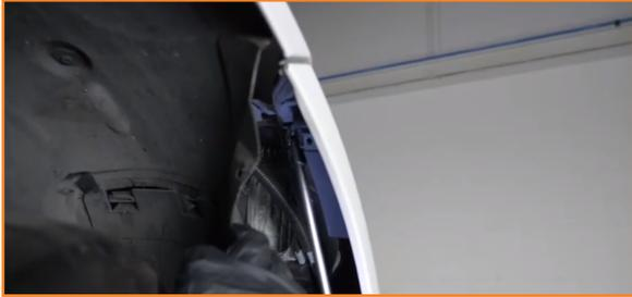
5. With the liner back, separate the window washer quick-disconnect within the wheel well. Slide the black tab back to release the connection.
