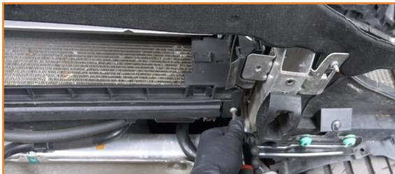
16. Release the heat exchanger and lower it out of the vehicle.
