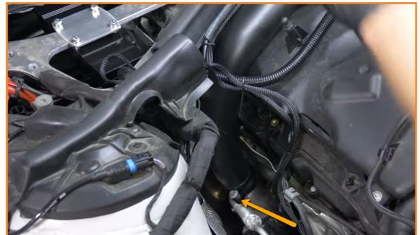
14. Attach a silicone coupler to the front intercooler pipe. Then set the front pipe and slide the coupler onto the intercooler.
