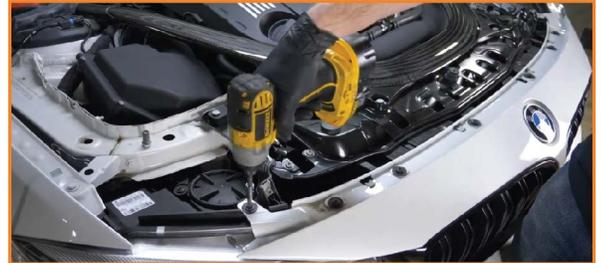
3. Remove all the bolts on the lower splash shields and wheel well liners. (25x 8mm bolts, 2x 13mm bolts)
