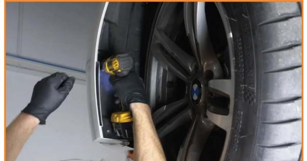
4. Pull back the wheel well liner to gain access behind it. Remove the bolts that secure the bumper to the edge of the fender. (4x 8mm bolts)
