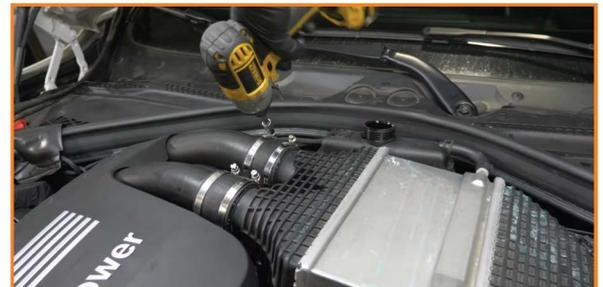
4. Separate the quick-disconnects from the intercooler. Lift the clip on each one to free the connections. Place something underneath to catch residual fluid from these connections. (3x spring clips)
