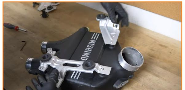
11. Transfer the temperature sensor to the Mishimoto intercooler using the provided hardware. (2x M5 3mm Allen bolts)
