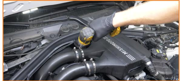
11. Pull away and up to remove each intercooler pipe.
