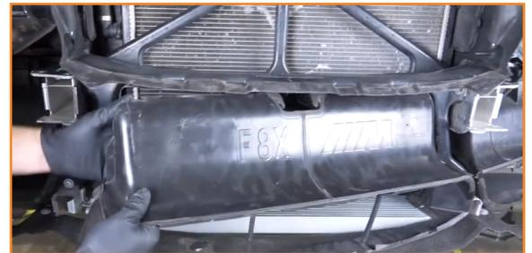
12. Remove the bolts that secure the cross brace and slide it out from behind the upper ducting. (6x T45 torx)
