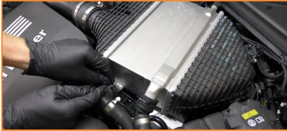
5. All connections to the intercooler at this point should be loose. Lift the cold side, and then slide the intercooler out at an angle.
