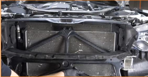
13. Separate the quick-disconnects along the passenger side of the heat exchanger.
