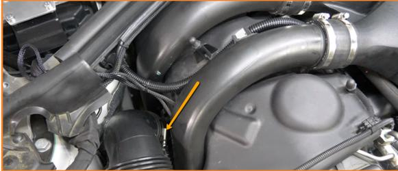
7. Disconnect the MAF sensor. Depress the black tab at the center to release the connection. Then lift the airbox out of the way.
