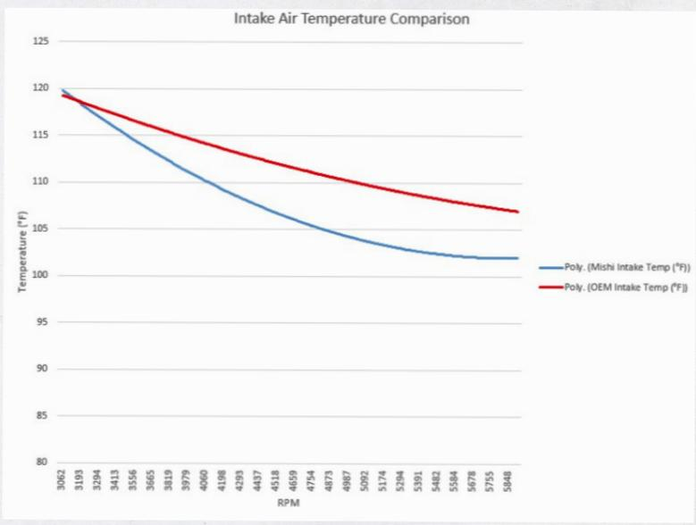
**Figure 8:** Comparison of stock and Mishimoto intake air temperatures
