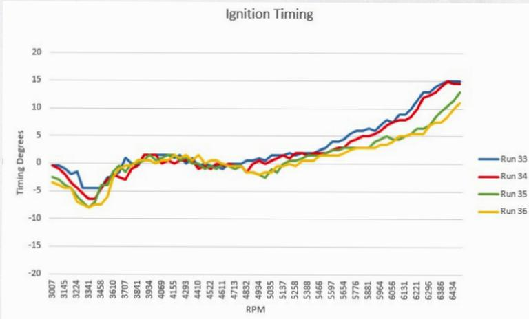
**Figure 4:** Ignition timing is pulled as the ECU tries to learn itself.
