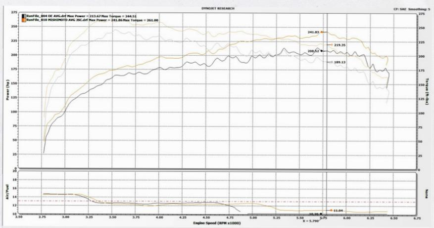
**Figure 3:** Gains of approximately 28 whp and 16 wtq are seen when the Mishimoto Intake is compared to the stock intake.
