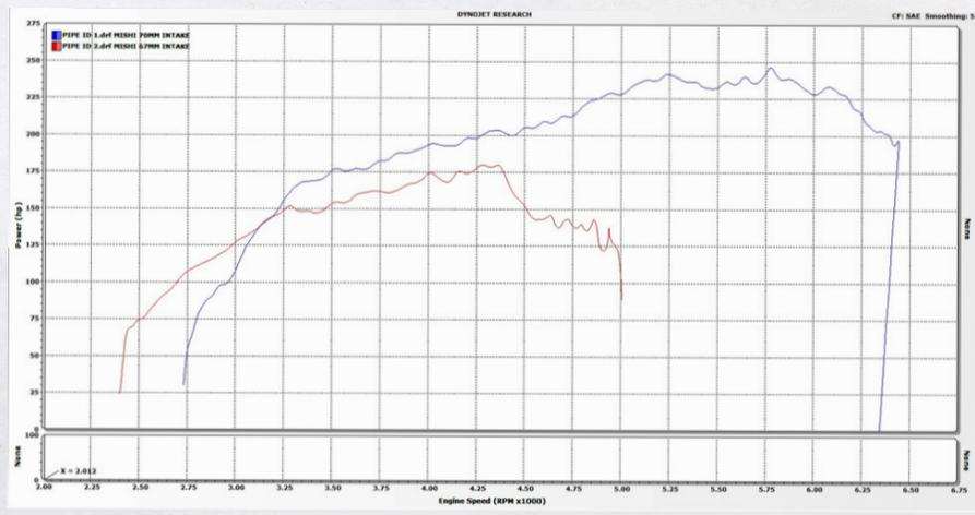
**Figure 2:** Comparison between the selected pipe prototype (blue) and a rejected prototype. The rejected prototype caused the WRX to run so poorly that the run had to be stopped before redline.
