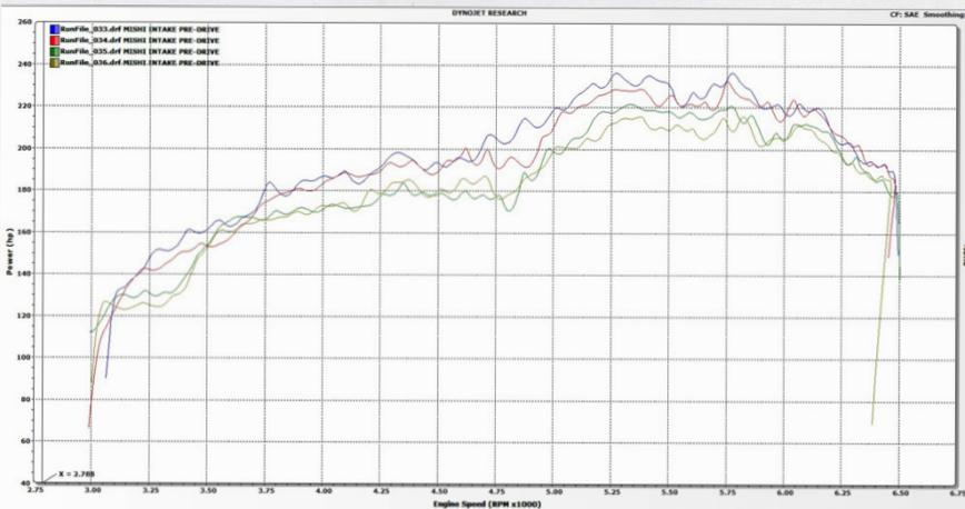
**Figure 5:** This decrease in ignition timing leads to a decrease in overall power.
