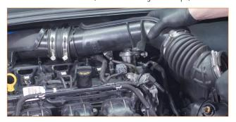
13. Separate the airbox from the vehicle by lifting it upward. The airbox is held in with three studs and grommets.
