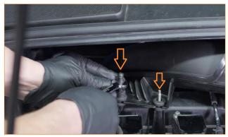
12. Loosen the two worm-gear clamps that secure the lower intake tube to the airbox and upper intake tube. Then remove the lower intake tube. (2x 7mm worm-gear clamps)
