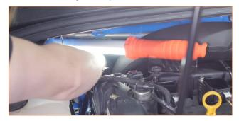
15. Separate the upper intake tube from the turbocharger, lift it off the mounting studs and rotate it to access the hose connected to the back of the tube. Disconnect this hose by squeezing the knurled tabs.
