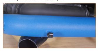
29. Remove the metal insert and rubber grommet from the stock intake tube. Transfer the insert and grommet to the bracket included with your kit. Then install the bracket to the Mishimoto induction pipe with the included bolt as shown here. Leave the bolt loose for now. (1x 10mm bolt)
