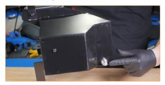
03. Locate the mounting bracket with a round cutout in your kit. Install this bracket to the airbox just below the air inlet duct. The tab on the bracket will fit into a slot on the airbox. Tighten this bolt completely. (1x 4mm Allen bolt, 1x lock washer, 1x metal washer)
