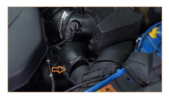
08. Separate the tree clip that secures the harness to the airbox, and disconnect the harness from the sensor.
