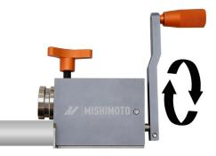
**5.** As you rotate the handle, gradually tighten the top knob in half-turn increments. This will increase the pressure on the rollers and create a more defined bead.
