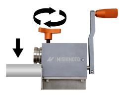
**3.** Rotate the top knob clockwise until the rollers touch the pipe. Tighten the knob approximately half a turn to clamp the pipe in place.
