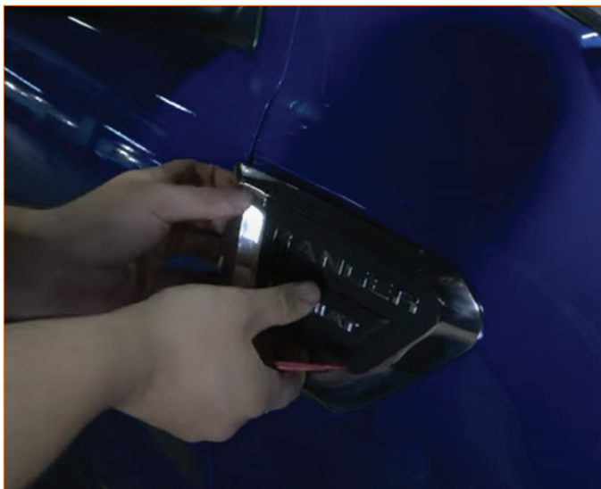
04. Cut inner fender using template.
