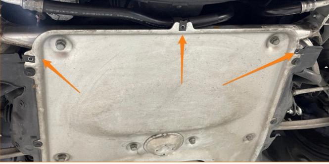
5. Remove 6x screw clips from the factory oil cooler skid plate and install them in the locations shown.
