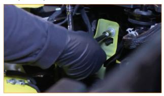
**14.** Remove the tree clips from the harness on the bottom of the wheel well. (flathead screwdriver)
