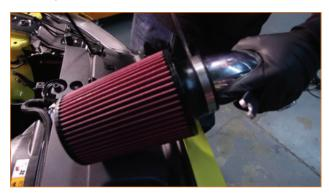
**21.** Attach the upper rubber bushing to the intake pipe. The unused threads must be facing upward. [10mm ratchet wrench]
