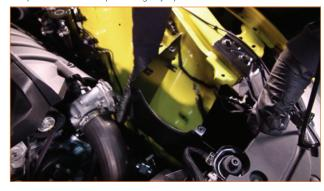
**17.** Make sure that the tab on the airbox falls in line with the ground bolt, and fully tighten the 8mm ground bolt.
