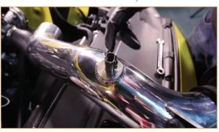
23. Attach the large worm-gear clamp to the hose.
