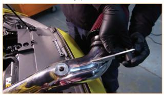
**22.** Reinstall the IAT sensor by pushing on the opening of the pipe and then turning clockwise until it stops. Gently pull upward to be sure that the IAT sensor is seated correctly.
