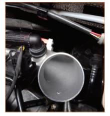
8. Reinstall the air intake tube. (1x worm gear clamp, 1x spring clamp)
