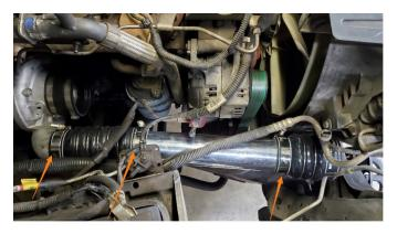
6. Place shop towels or a container under the transmission cooler line connections to catch the fluid that will leak out. Then, remove the dust covers from the transmission cooler line connections and disengage the connections. Properly dispose of any transmission fluid.
