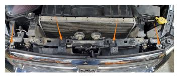
13. Install the Mishimoto boots and intercooler piping onto the vehicle with the supplied clamps, as shown below.
