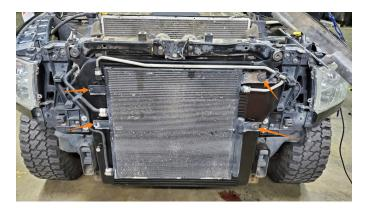
11. Transfer the rubber grommets from the stock intercooler to the Mishimoto intercooler and install the supplied metal shroud with the two (2) supplied M6 x 16mm bolts, as shown below.
