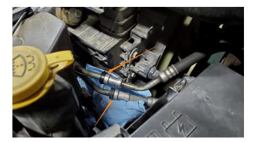
16. Reconnect the transmission cooler lines and reinstall the dust caps onto the fittings. Then, replace the seals at the A/C condenser line junction with new seals and reconnect the A/C condenser lines with the two (2) bolts removed in step 5. The bolt that mounted the junction to the stock intercooler will not be reused. (Image on right)
