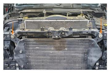
3. Remove the four (4) bolts securing the grille to the vehicle. Then, remove the grille from the vehicle by pulling it away from the vehicle to disengage the clips securing the bottom.
