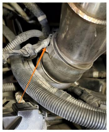
**5. BE SURE THE REFRIGERANT HAS BEEN PROPERLY RECOVERED BEFORE PREFORMING THIS STEP.** Remove the two (2) bolts securing the junction of the A/C condenser lines. Then, remove the one (1) bolt securing the junction to the intercooler.
