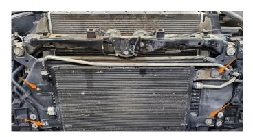
17. Reinstall the bumper, plastic shrouds, & grille by reversing the removal steps. Check the transmission fluid level before driving the vehicle and top off if needed. The A/C system can be recharged by most mechanics. The installation is now complete.
