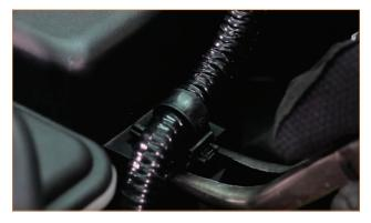
05. Release the clip that secures the coolant overflow hose to the top of the airbox.
