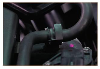
06. Remove the bolt that secures the airbox to the radiator support next to the coolant overflow reservoir. (1x 10mm bolt)
