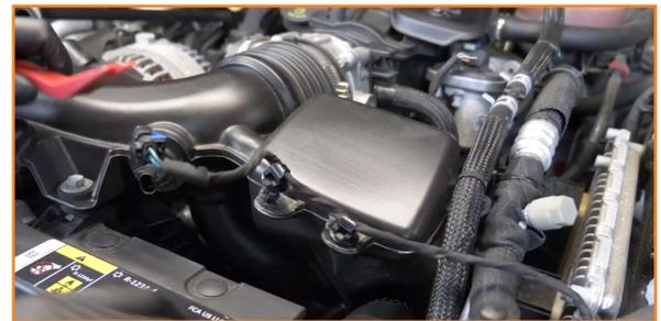
3. Remove the bolts that secure the front of the intake tube to the radiator cover. (2x 10mm bolts)
