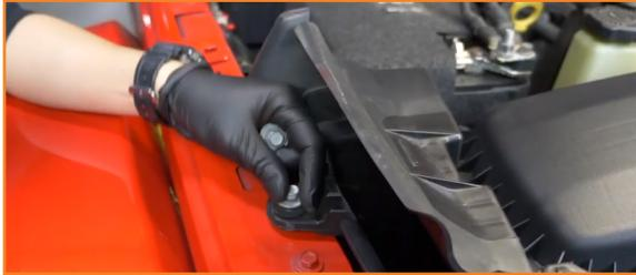
5. Loosen the clamps on each end of the intake tube. (2x worm gear clamps)
