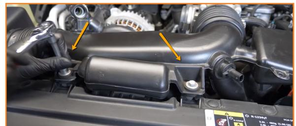
4. Remove the bolt that holds down the airbox. (1x 10mm bolt)
