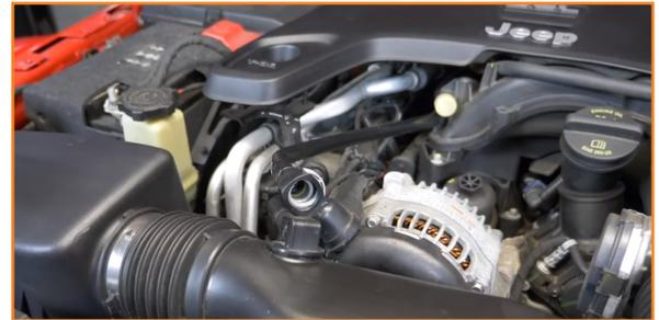
2. Disconnect the intake air temperature sensor from the intake tube. Release its wiring harness. One clip is linked to a nearby coolant hose. (3x tree-clips)
