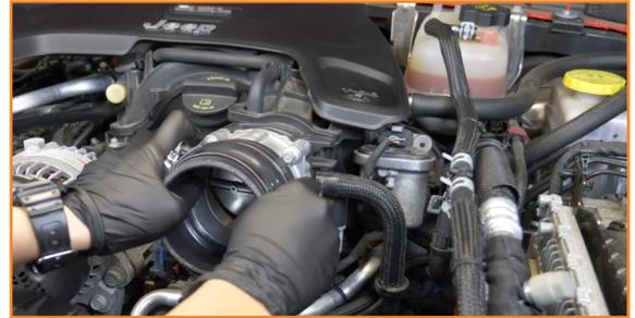
13. Install the intake tube to the coupler and airbox. (2x worm gear clamp)
