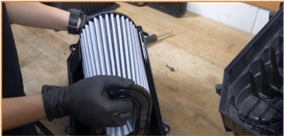
9. Attach the Mishimoto airbox lid and filter to the bottom half. (4x 8mm screws)
